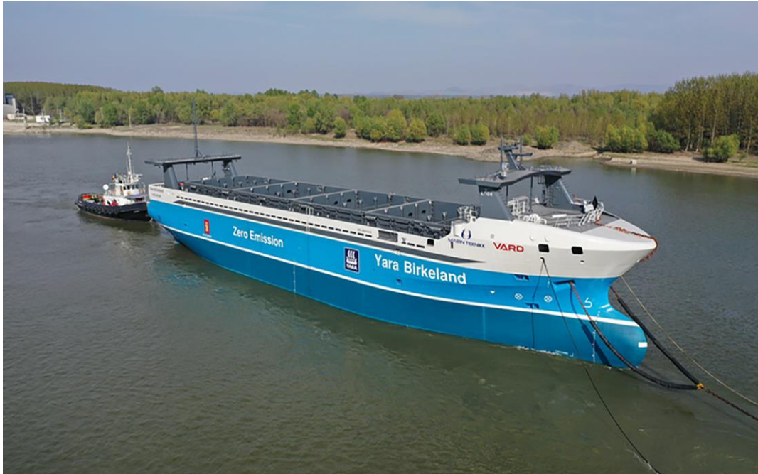
Figure 8 - The Yara Birkeland, a fully autonomous electric container barge, is deployed in Norway, November 2021. Such vessels provide clean propulsion and are aided by the latest and most advanced methods for navigation. Source: Engadget
